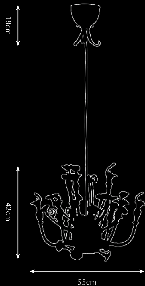
Itemnr: PA 950 Model: CarniForest hanging lamp Material: Casted Brass Sockets: 9x G4 LED + GU5.3 LED spot Finishes: Natural brass , Dutch silver
